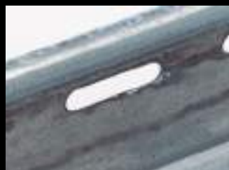
Acabado HR a 3000 horas HR coating at 3000 hours
